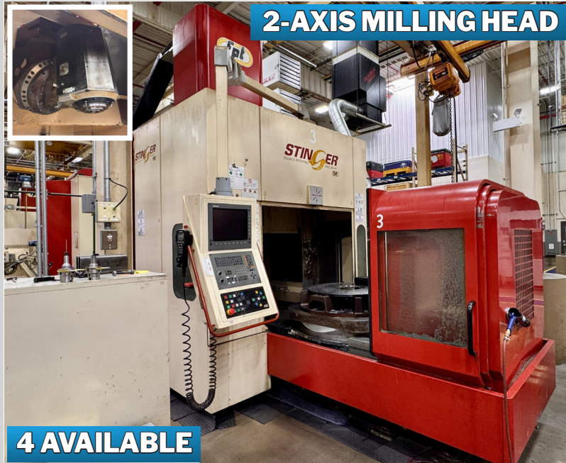
FPT STINGER 5-AXIS CNC BRIDGE-TYPE VERTICAL MACHINING CENTER
