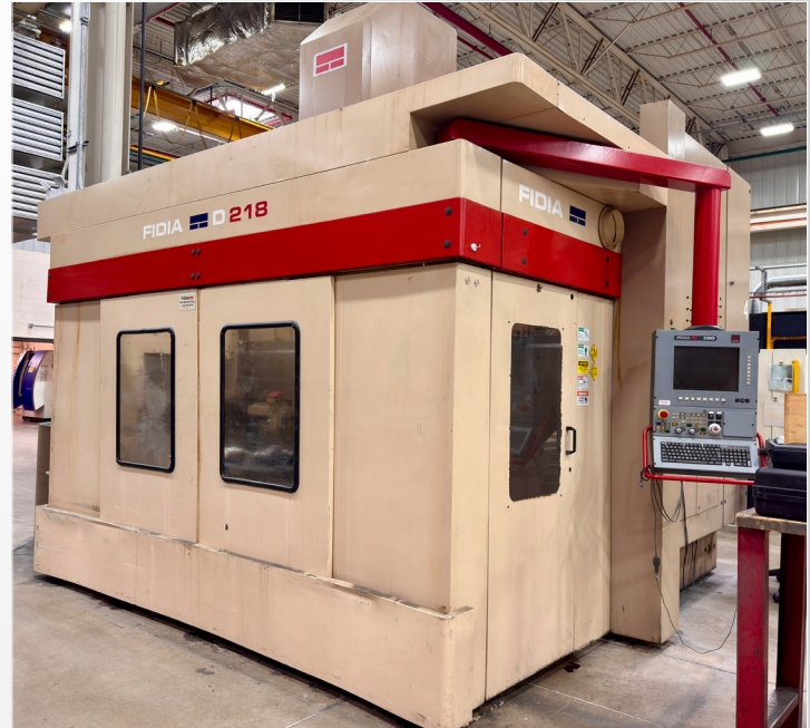
FIDIA D218 CNC 5-AXIS BRIDGE-TYPE VERTICAL MACHINING CENTER
