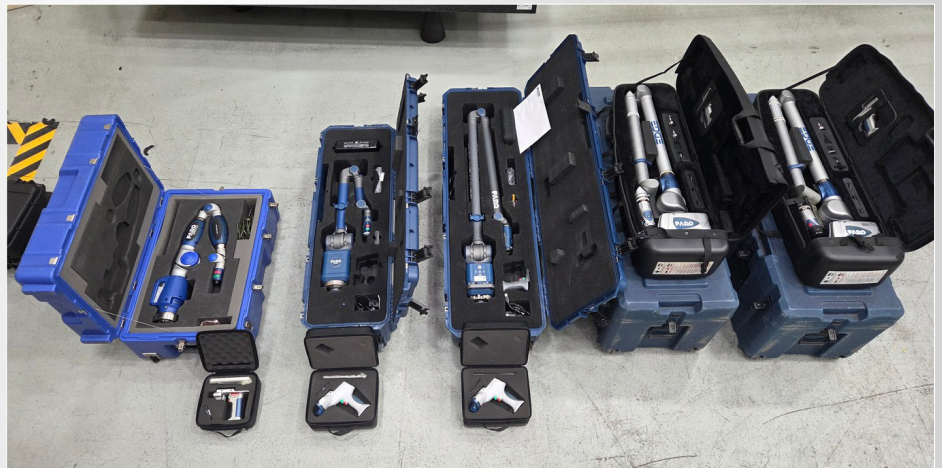
VIEW OF FARO PORTABLE CMMs
