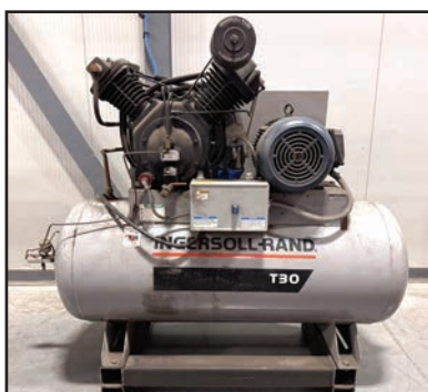
INGERSOLL RAND 15 HP AIR COMPRESSOR
