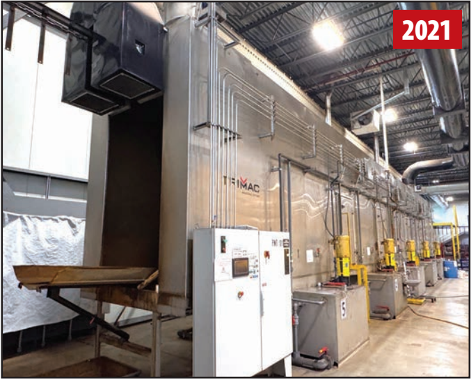
TRIMAC KEMAC STAINLESS STEEL 5-STAGE WASH
