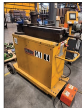
2015 BAILEIGH/RUSCH M325 PROGRAMMABLE ROTARY DRAW BENDER
