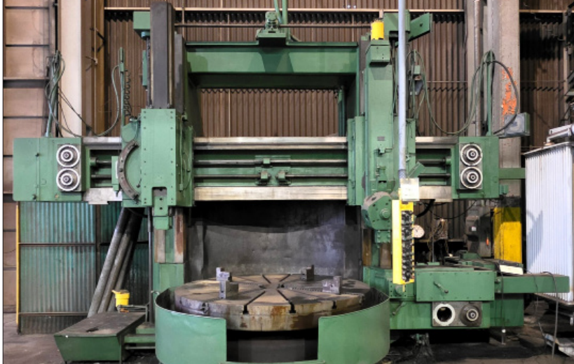
GRAY 84" VERTICAL BORING MILL VIEW LOT #47
