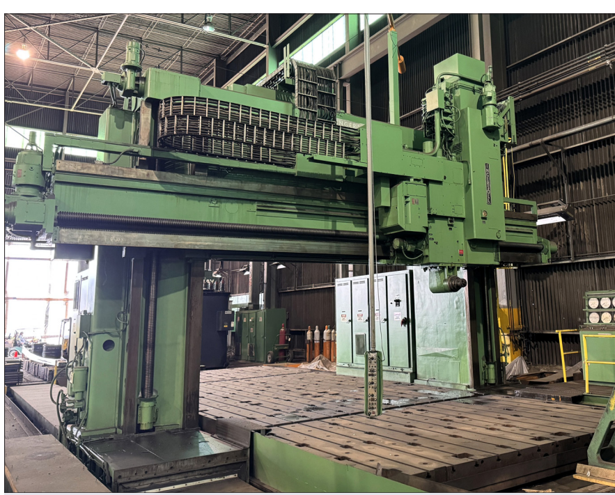
INGERSOLL 17' X 10' X 47' DOUBLE HOUSING TRAVELLING GANTRY PLANER MILL
