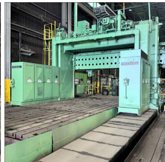
INGERSOLL 17' X 10' X 47' DOUBLE HOUSING TRAVELLING GANTRY PLANER MILL
