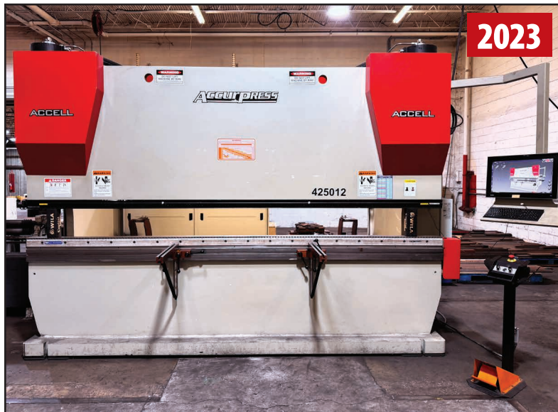
ACCURPRESS 250 TON X 12' CNC BRAKE
