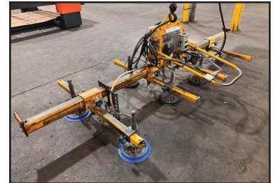
ANVER ELECTRIC VACUUM SHEET LIFTER
