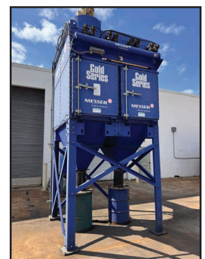
MESSER FUME FILTER EXHAUST SYSTEM
