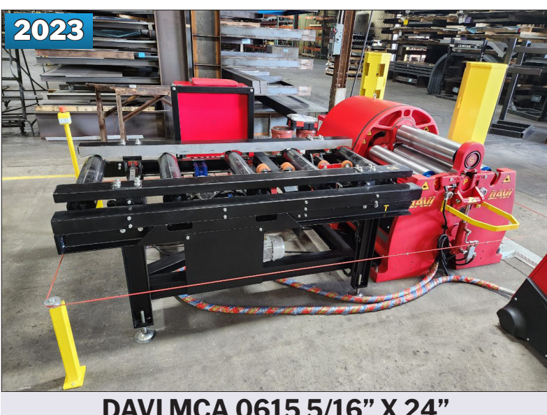
DAVI MCA 0615 5/16" X 24" 4-ROLL HYDRAULIC PLATE ROLL
