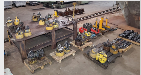
VIEW OF LIFTING MAGNETS
