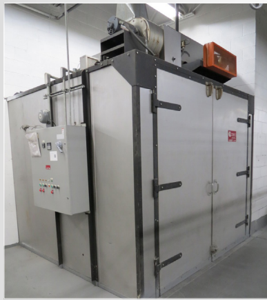
GEHRICH 2-DOOR PASS THROUGH 700 MBTU OVEN
