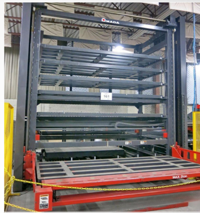
AMADA AUTOMATION 6-SHELF TOWER MATERIAL LOADER
