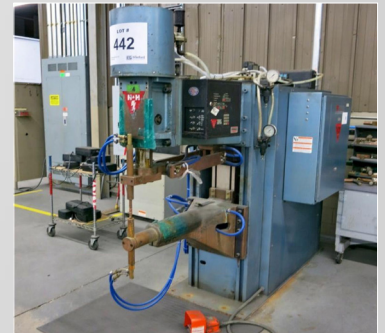
H&H PMC02ST 200 KVA DEEP THROAT SPOT
