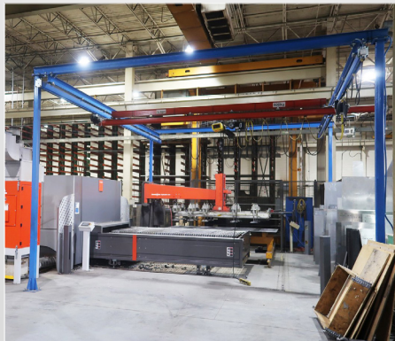
DYTAN TYPE 2002 CANTILEVER MATERIAL STORAGE AND DELIVER SYSTEM ½ TON OVERHEAD CRANE SYSTEM
