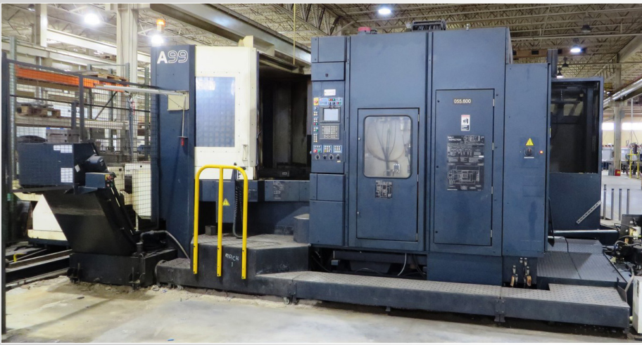
MAKINO A99 CNC HORIZONTAL MACHINING CENTER WITH 12-STATION FMS SYSTEM LOAD/UNLOAD
