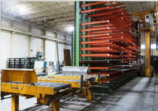
DYTAN TYPE 2002 CANTILEVER MATERIAL STORAGE AND DELIVER SYSTEM ½ TON OVERHEAD CRANE SYSTEM
