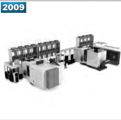
2009 MAZAK HORIZONTAL MACHINING CELL CONSISTING OF (2) MAZAK HCN-6800-II CNC HORIZONTAL MACHINING CENTERS
