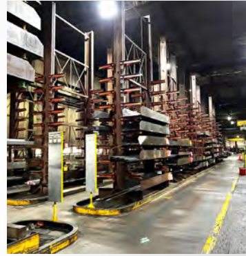
VIEW OF CANTILEVER RACKING
