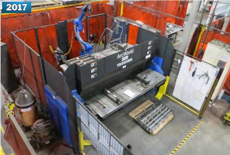
YASKAWA MOTOMAN MA2010 WELD CELL WITH 6-AXIS ROBOT & FERRIS WHEEL POSITIONER
