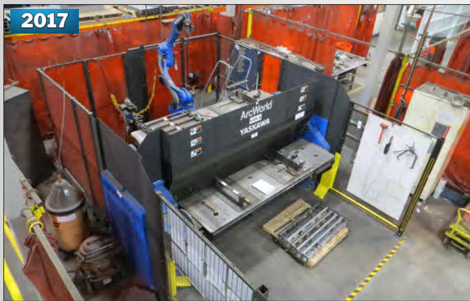
YASKAWA MOTOMAN MA2010 WELD CELL WITH 6-AXIS ROBOT & FERRIS WHEEL POSITIONER
