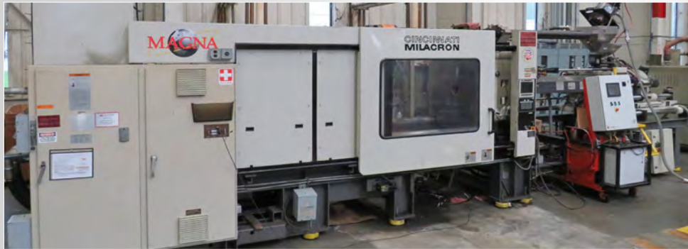
CINCINNATI MILACRON MODEL MH-725-95, 725-TON X 95 OZ. CNC HYDRAULIC INJECTION MOLDING MACHINE
