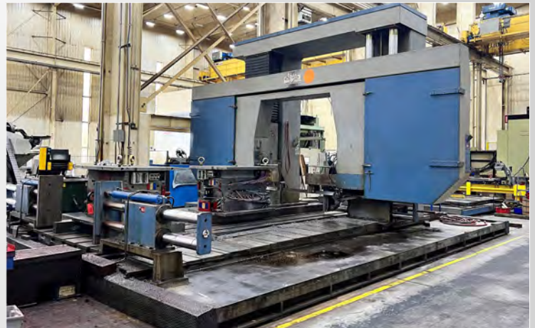
FABBRICA ITALIANA SEGATRICI MODEL 2000.P LARGE CAPACITY GANTRY TYPE HORIZONTAL BAND SAW
