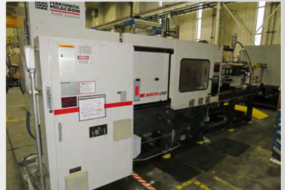
FERROMATIK-MILACRON "MAGNA 250" MODEL MH25021, 250-TON X 21 OZ. SHOT CAPACITY HYDRAULIC CLAMP HORIZONTAL RECIPROCATING SCREW PLASTIC INJECTION MOLDING MACHINE
