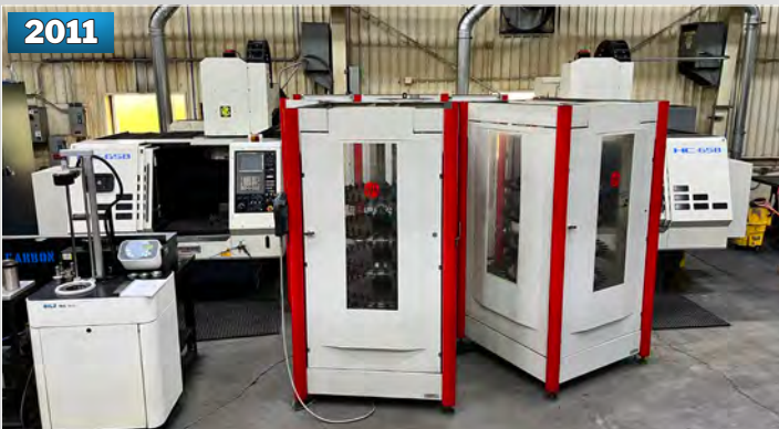
2011 (2) ROKU-ROKU-SANYO HC-658 4-AXIS HIGH SPEED CNC VERTICAL MACHINING CENTERS
