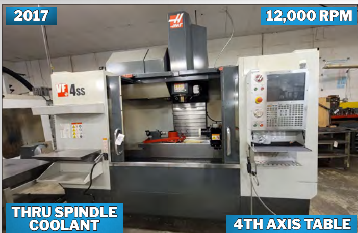
HAAS VF-4SS VERTICAL MACHINING CENTER
