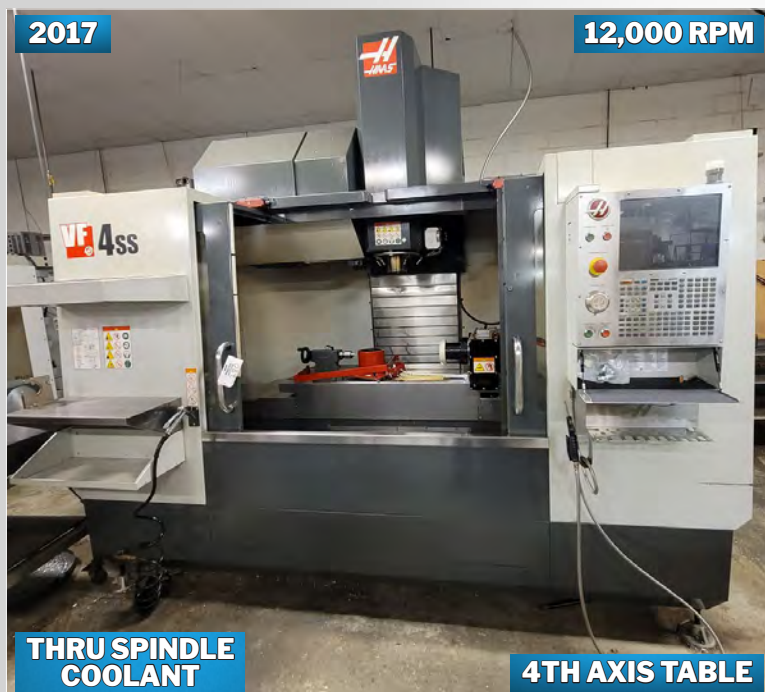
HAAS VF-4SS VERTICAL MACHINING CENTER
