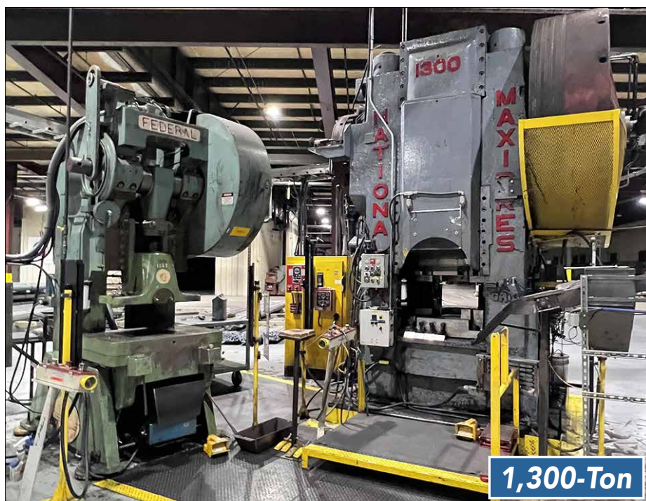
National 1300 Maxipress 1300-Ton Forging Press & Federal OBI Press
