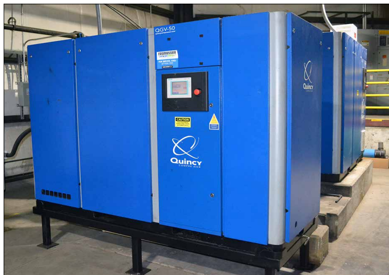
Quincy QGV-50A 50-HP Rotary Screw Air Compressor
