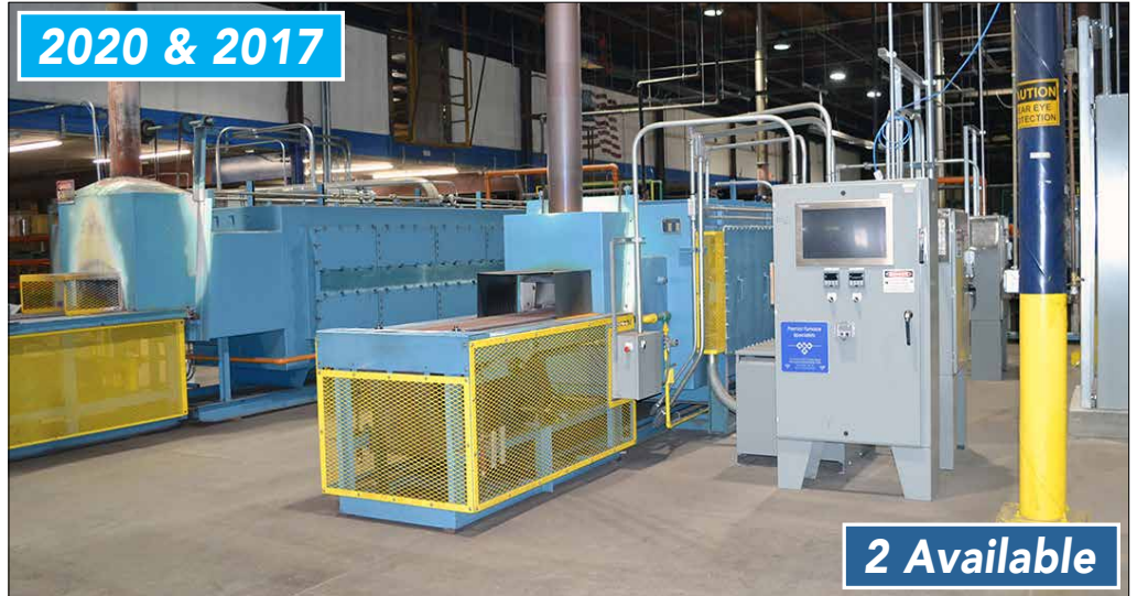
Premier Furnace Specialists 20 x 8 Continuous Mesh Belt Electric Brazing/Annealing Furnaces
