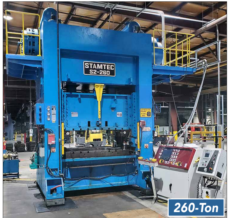
Stamtec S2-260 260-Ton Straight Side Mechanical Double Crank Press
