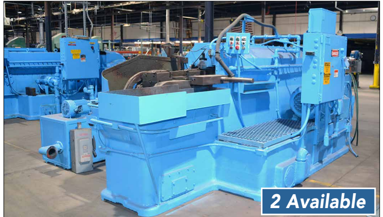
Foote-Burt 15-Ton x 110" Horizontal Hydraulic Broaching Machine
