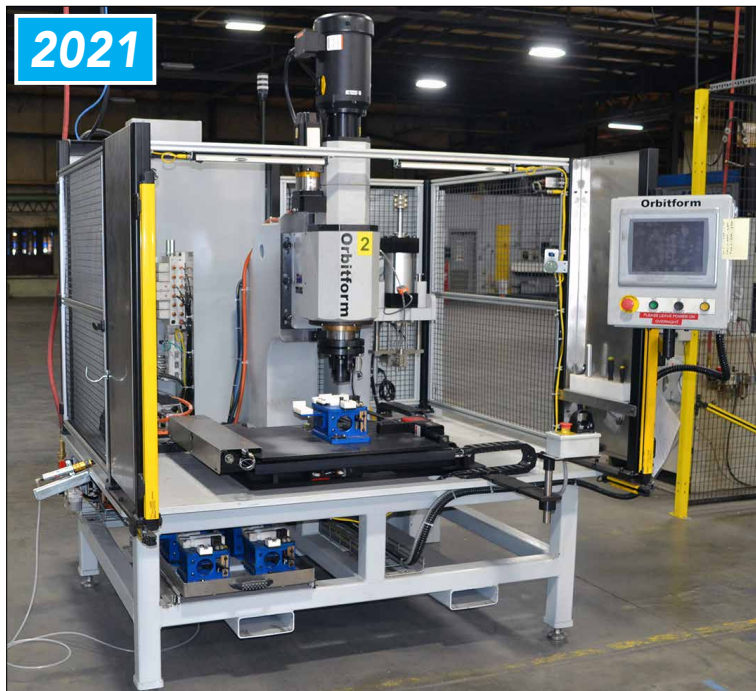
Orbitform CNC Orbital Riveter
