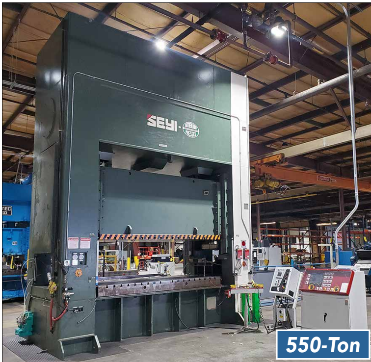
Seyi Sutherland HSD-550 550-Ton Straight Side Mechanical Press
