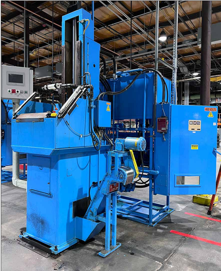
Broaching Machine Specialties VTF 10-66 10-Ton x 66" Twin Ram Vertical Hydraulic Broaching Machine
