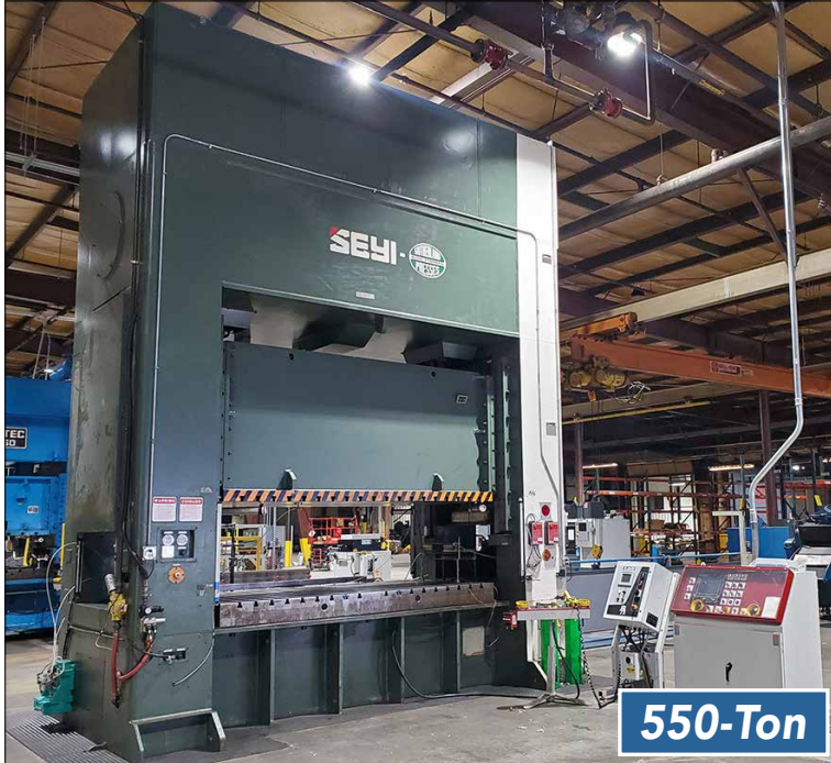
Seyi Sutherland HSD-550 550-Ton Straight Side Mechanical Press
