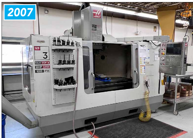
Haas VF-3B CNC Vertical Machining Center
