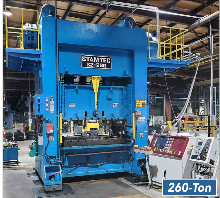
Stamttec S2-260 260-Ton Straight Side Mechanical Double Crank Press
