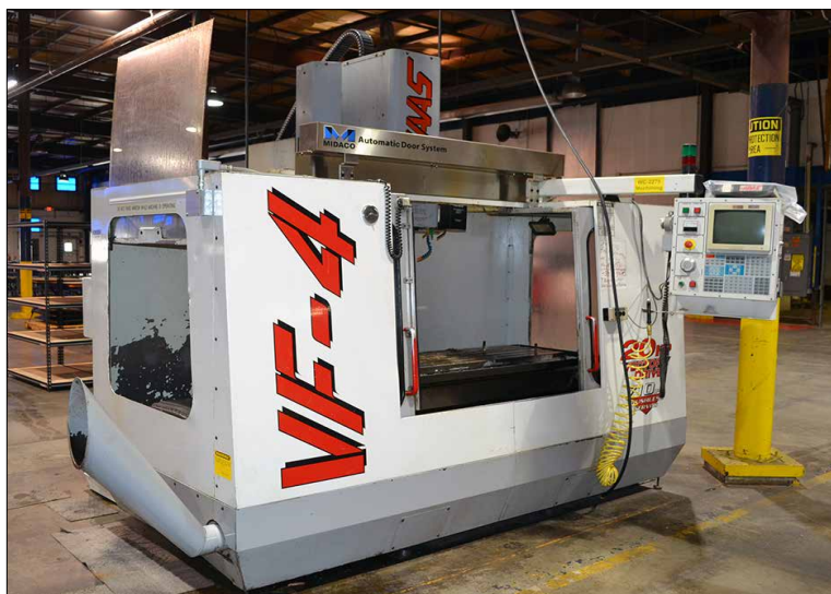
Haas VF-4 CNC Vertical Machining Center
