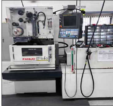
Fanuc Alpha-oic CNC Wire EDM
