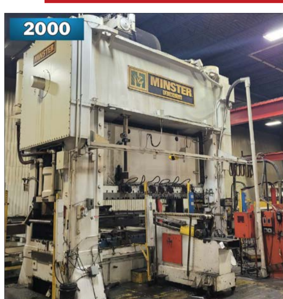
MINSTER E2-1000-144 HEVI-STAMPER TWO POINT ECCENTRIC SHAFT, PROGRESSIVE DIE PRESS VIEW VIDEO / LOT #23
