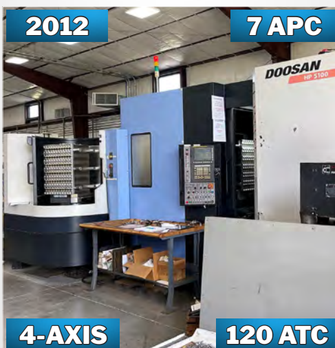
DOOSAN HP-5100 CNC HORIZONTAL MACHINING CENTER
