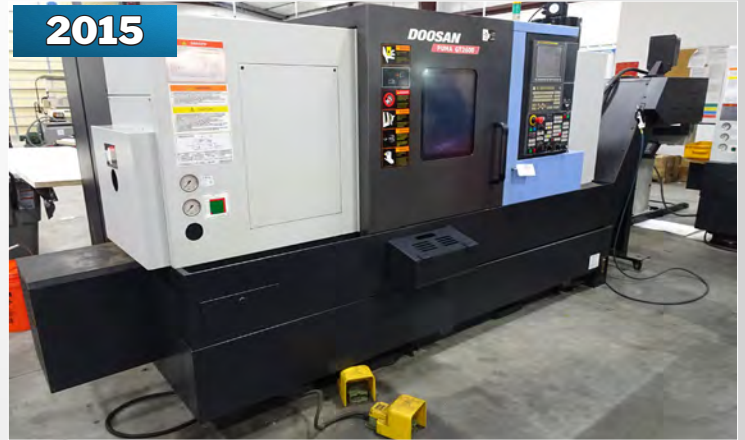
DOOSAN PUMA GT-2600 CNC TURNING CENTER
