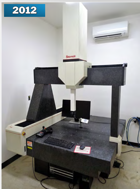
STARRETT RGDC 4040-24 COORDINATE MEASURING MACHINE
