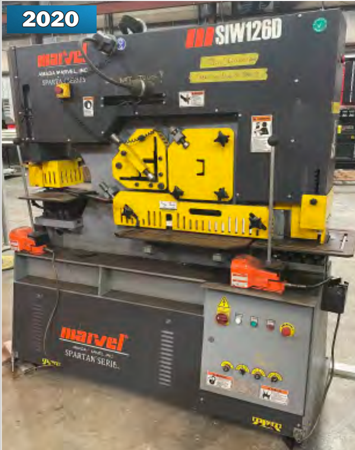
AMADA MARVEL MSIW126D-SPARTAN HYDRAULIC IRONWORKER
