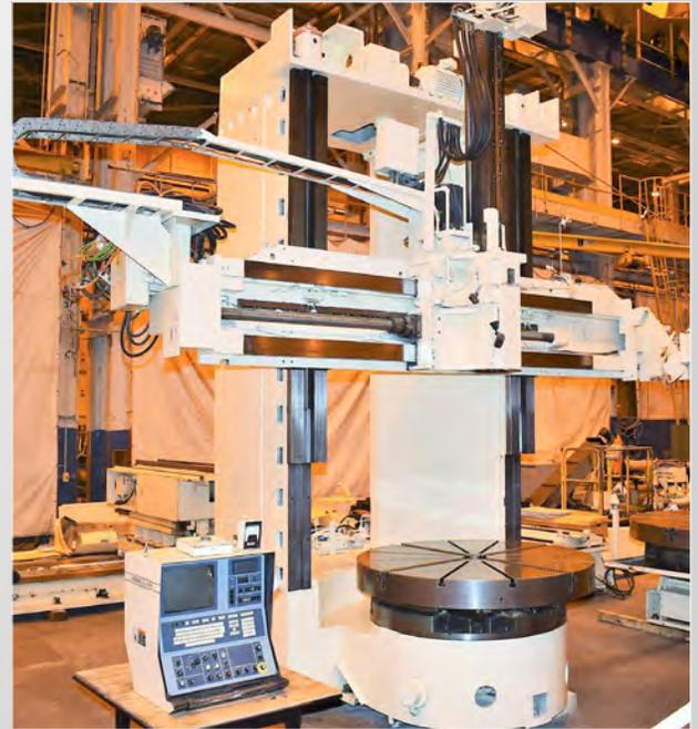
72" GIDDINGS & LEWIS HIGH COLUMN CNC VERTICAL BORING MILL
