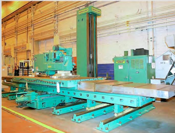
**GIDDINGS & LEWIS G60-T CNC TABLE TYPE HORIZONTAL BORING MILL**
