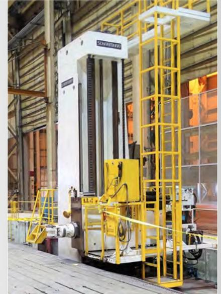
**SCHARMANN HEAVYCUT WFT-150 CNC FLOOR TYPE HORIZONTAL BORING MILL**
