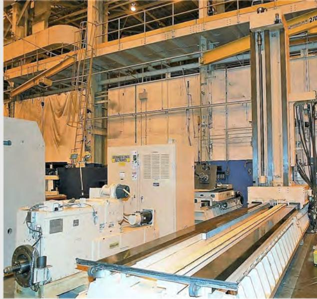
**GIDDINGS & LEWIS G60-FX CNC FLOOR TYPE HORIZONTAL BORING MILL**
