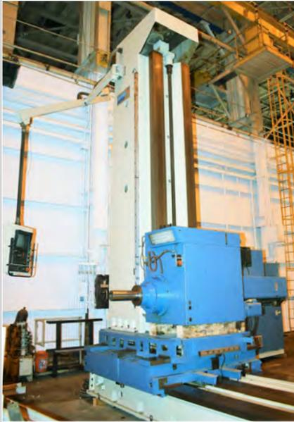
**UNION BFP130 CNC FLOOR TYPE HORIZONTAL BORING MILL**
