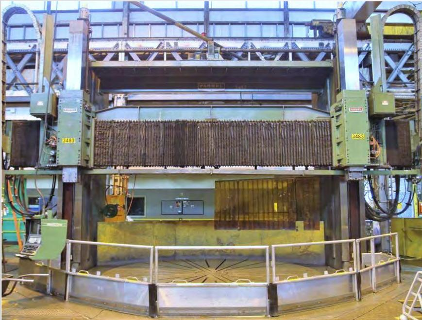
FARREL 192"/252" DOUBLE COLUMN CNC VERTICAL BORING MILL
