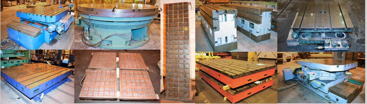
ROTARY TABLES, T-SLOTTED RISER TABLES, T-SLOTTED FLOOR PLATES, ANGLES & MAGNETIC TABLES
