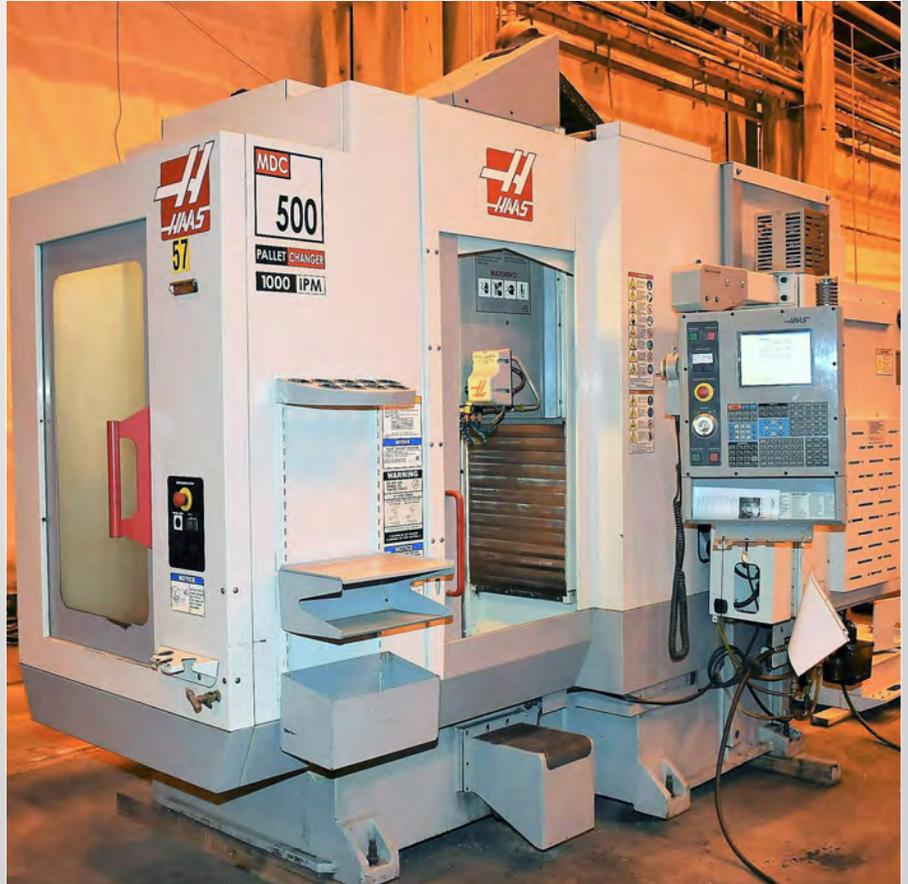
**HAAS MDC-500 CNC VERTICAL MACHINING CENTER WITH ROTARY PALLET CHANGER**
