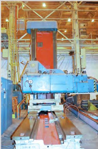
**SKODA WD 160B FLOOR TYPE HORIZONTAL BORING MILL**
