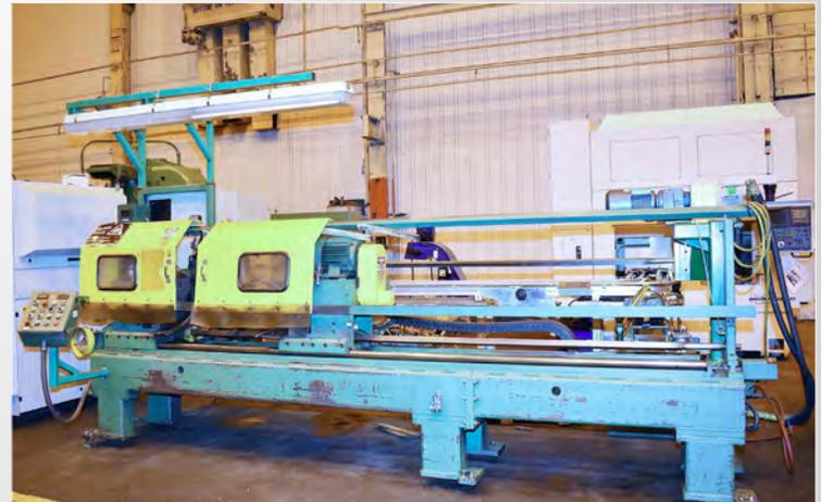
**HAVEN 912A DOUBLE END TUBE FINISHING MACHINE**
