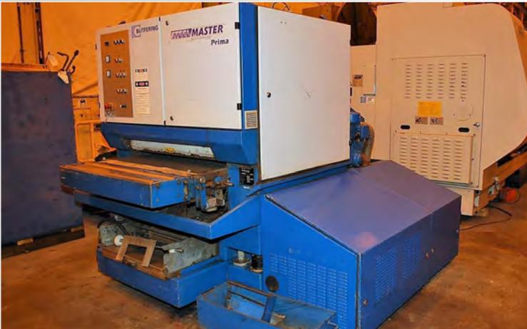
**STEELMASTER PRIMA W209-RD 37"WET DEBURRING & FINISHING MACHINE**
