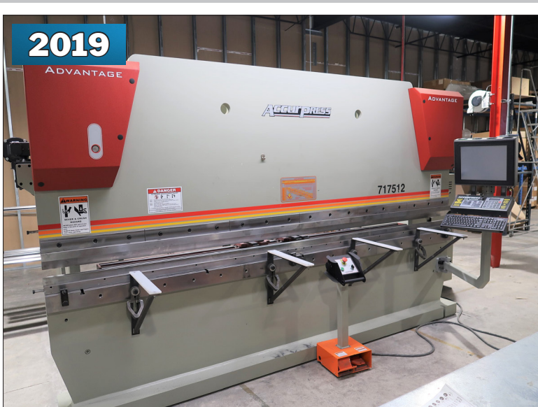
ACCURPRESS 717512 175 TON CNC PRESS BRAKE
