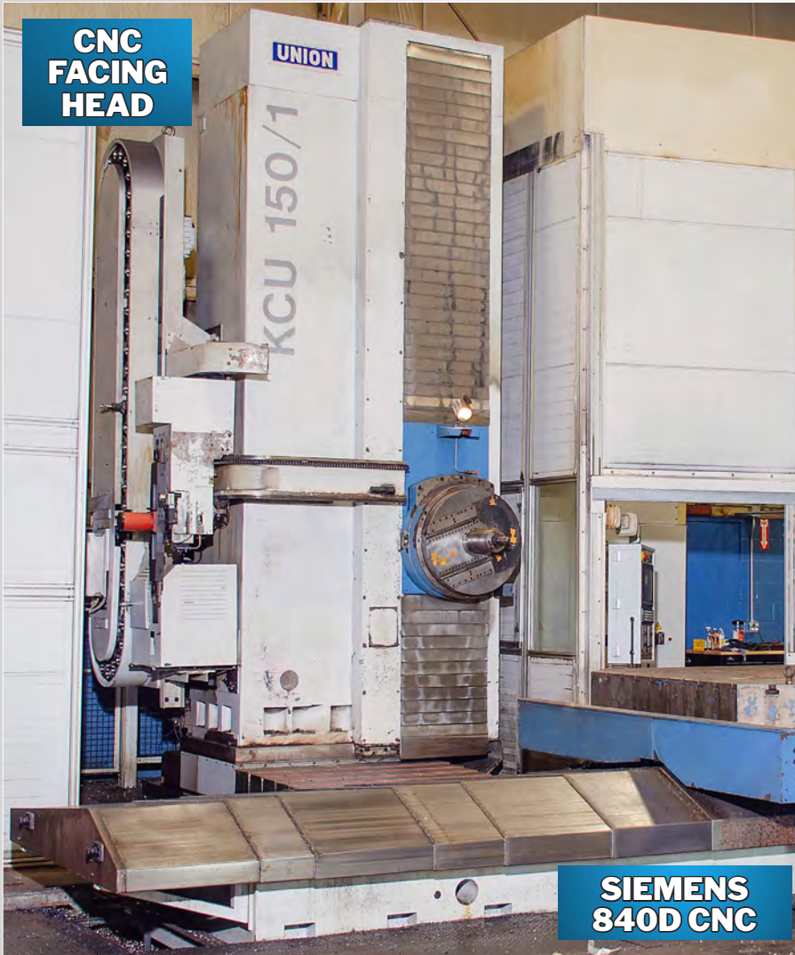
UNION KCU-150 HDT CNC HORIZONTAL BORING MILL
