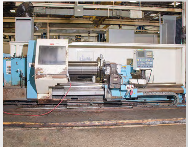
HANKOOK PROTEC 9NC 37" X 157" CNC LATHE
