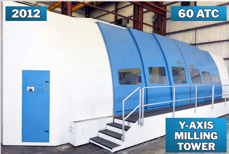
BOST T4F 79" X 354" CNC HORIZONTAL TURN/MILL LATHE
