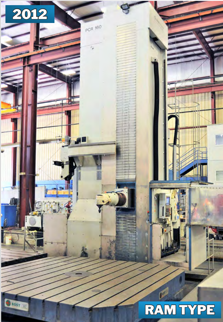
UNION PCR160 PLUS CNC FLOOR TYPE HORIZONTAL BORING MILL
