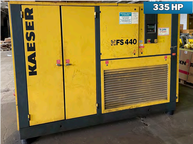
KAESER FS440 AIR COMPRESSOR
