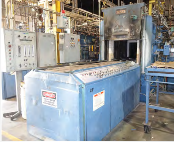
SELAS KARBO-MATIC PKMD-100-ERTNM-S GAS-FIRED QUENCH FURNACE
