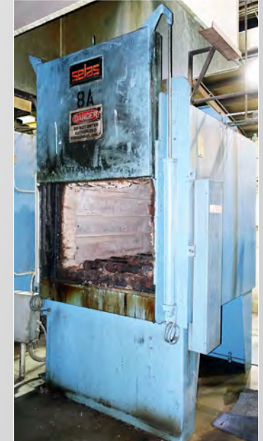
SELAS ELECTRIC FIRED BOX DRAW FURNACE
