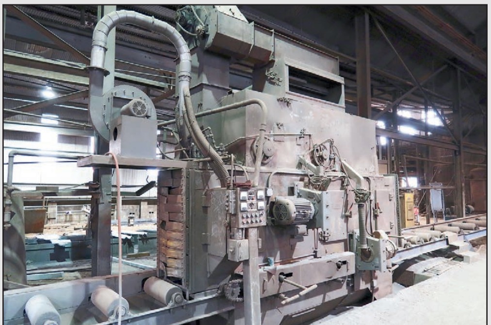
(4) Wheel Pass-Through Structural Steel Blast Units, 24" Wide x 48" High Opening, Shot Recovery and Delivery System, 65' Powered In-Feed Conveyor, 65' Powered Out-Feed Conveyor
