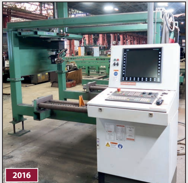
Peddinghaus Ocean Liberator SACM-1250A 5-Axis CNC Beam Coping Machine
