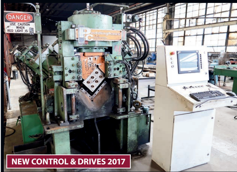
Peddinghaus AFCPS 823-B Angle, Flat Punch and Shear Line, 8" x 8" x 3/4" Angle Capacity
