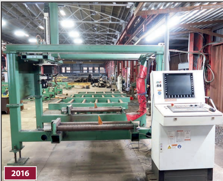
Peddinghaus Ocean Liberator SACM-1250A 5-Axis CNC Beam Coping Machine
