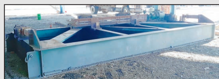
Cambro Model 500A Hydraulic Cambering and Beam Straightening Machine
