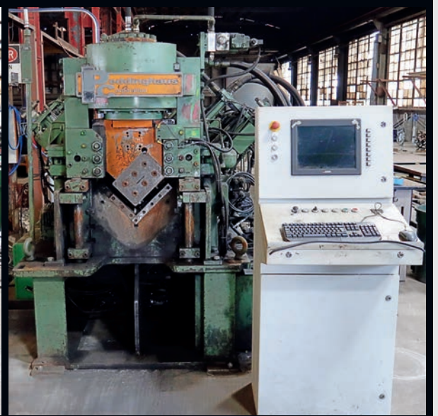
Peddinghaus AFCPS 823-B Angle, Flat Punch and Shear Line, 8" x 8" x 3/4" Angle Capacity
