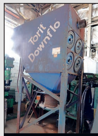
Torit Dust Collector
