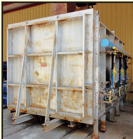
ERCO GAS FIRED CAR BOTTOM FURNACE
