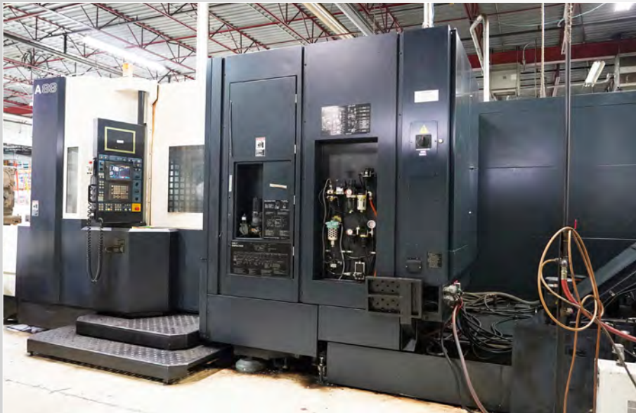
MAKINO TWIN PALLET HORIZONTAL CNC MACHINING CENTER
