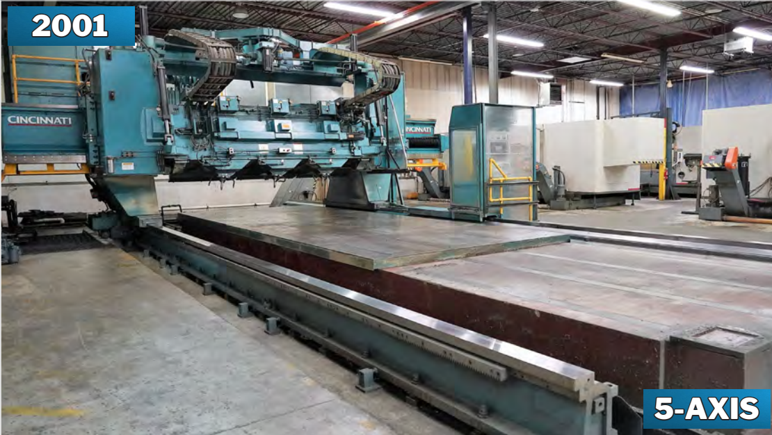
CINCINNATI "HIGH PERFORMANCE" 5-AXIS 3-SPINDLE CNC AEROSPACE GANTRY-TYPE PROFILER
