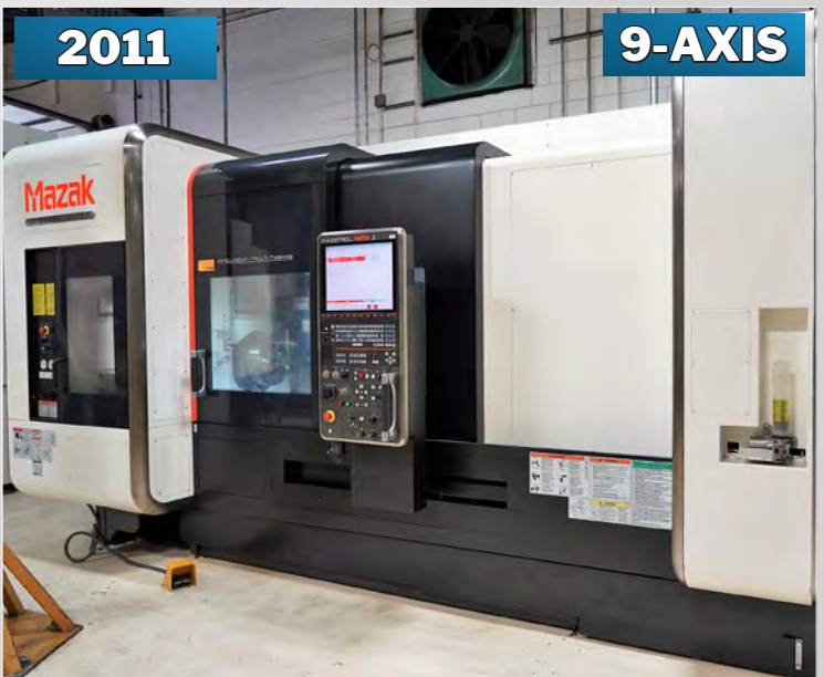
MAZAK INTEGREX i400-ST CNC 9-AXIS TURNING & MILLING CENTER
