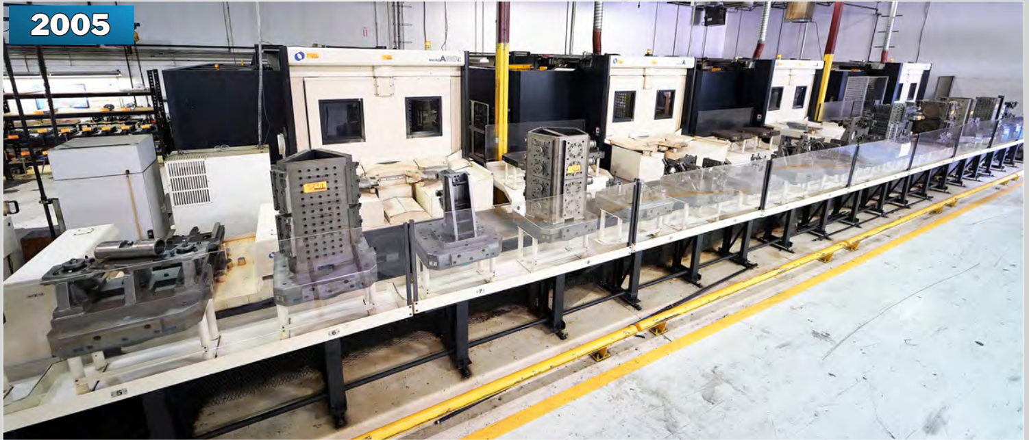
MAKINO A88/A88E LINE, 4 CNC HORIZONTAL MACHINING CENTERS WITH 32 PALLET SHUTTLE SYSTEM
