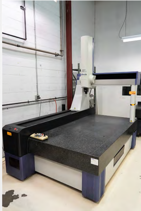
MITUTOYO CRT-A916 CRYSTAL APEX BRIDGE TYPE CMM
