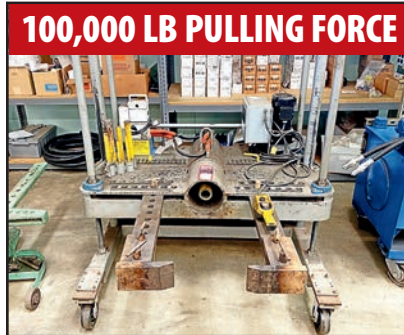
100,000 LB PULLING FORCE POULAN P-200 HYDRAULIC PULLER PRESS
