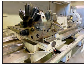
POREBA PNA-80/BARUFFALDI 8-POSITION TURRET, TAILSTOCK AND STEADY RESTS
