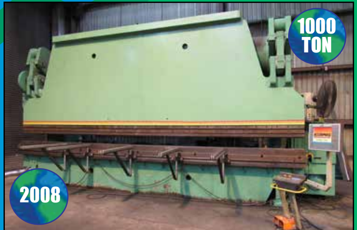
1000 TON X 24' ACCURPRESS 7-AXIS CNC HYDRAULIC PRESS BRAKE
