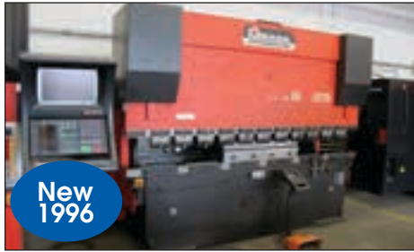
AMADA PROMECAM CNC 8' X 88-TON PRESS BRAKE MODEL HFBO-8025; 5 AXIS CNC BACK GAUGE
