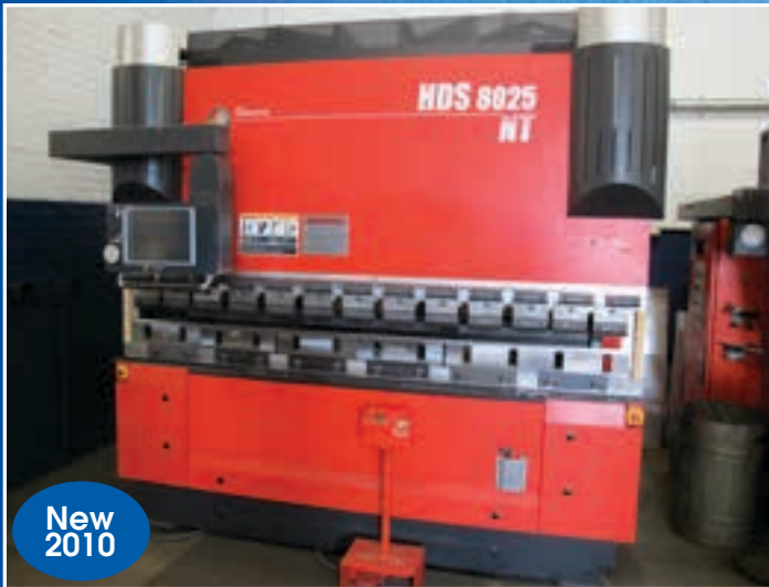
Amada Promecam CNC, 8' x 88-Ton Press Brake Model HDS-8025-NT, 5-Axis, Back Gage
