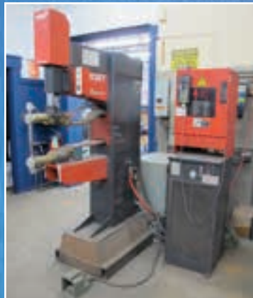
AMADA METRICS SPOT WELDER MODEL ID-40-ST, 95 KVA
