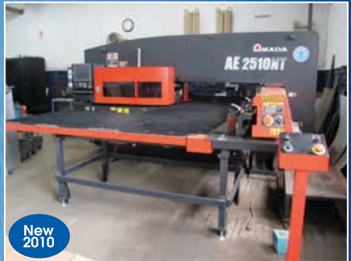
Amada Electric Servo CNC Turret Punch Model AE2510NT, 22-Ton, 51-Station Turret
