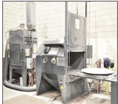
CANABLAST DCM-160 blast cabinet with rotary table and media recovery
