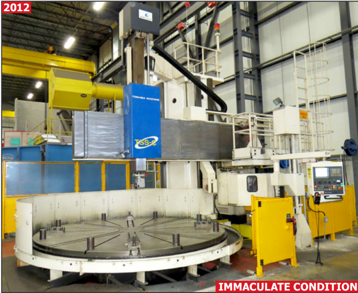
TOSHIBA TSS 40/67C, travelling column CNC open side vertical boring & live milling center
