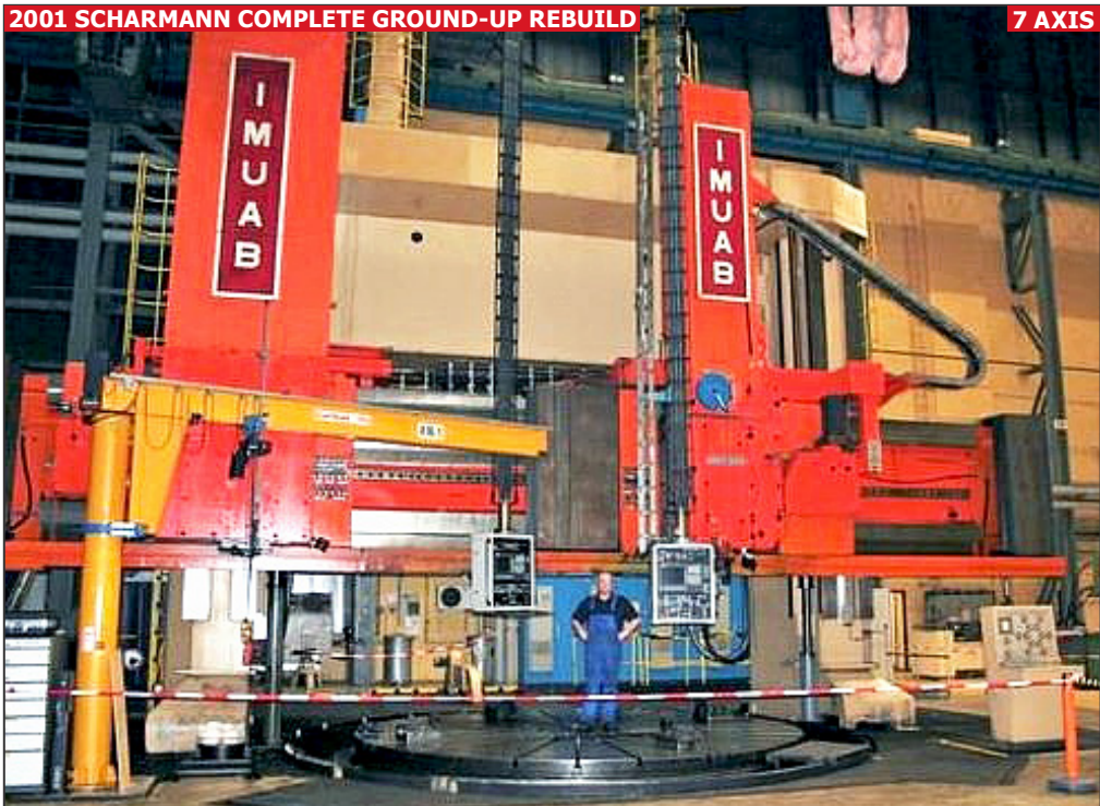
TITAN IMUAB SC 50/67, 7-axis CNC vertical boring mill and live milling center
