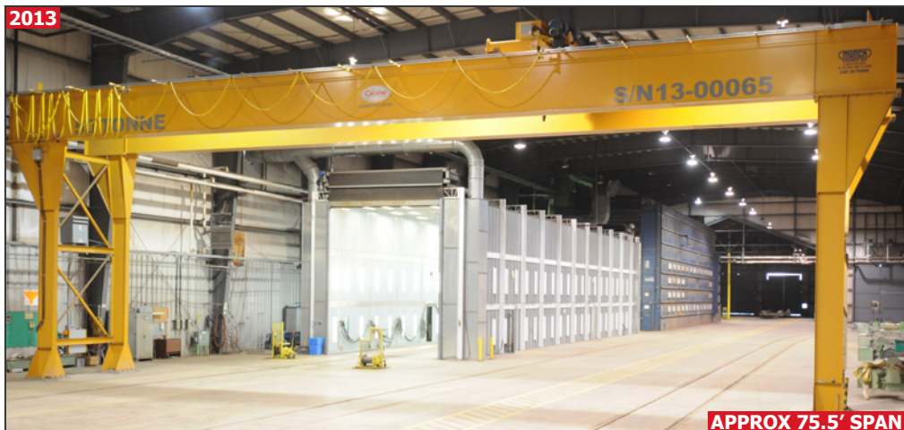
View of MUNCK 50 TON capacity free standing double girder overhead crane & very late model, heavy capacity paint shop
