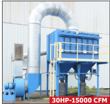
CINCINNATI FAN HDBI – 300 CJP 36 cyclonic type dust collector
