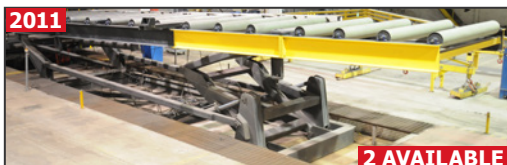
DAVI 46' x 10' hydraulic scissor lift type powered in feed table
