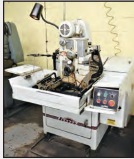
SUNNER MBC-1805-D HONE WITH POWER STROKE
