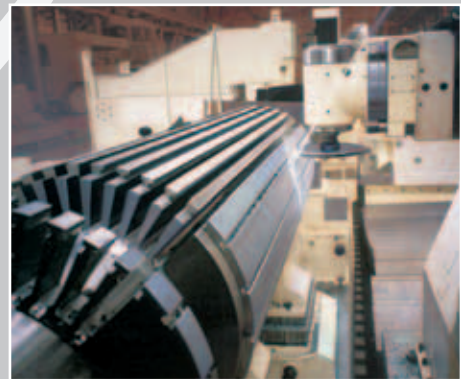
Workstation including a special headstock and manipulator for milling of turbogenerator rotor slots.
