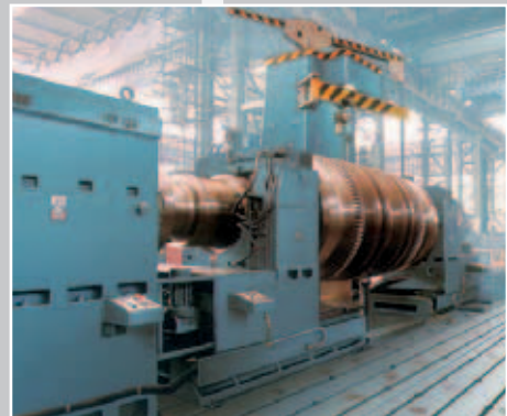
Workstation equipped with rotary manipulator for machining of steam-turbine rotor shafts.
