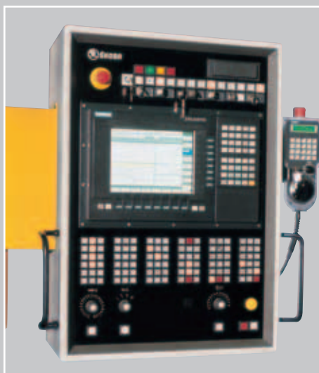
Main control panel SIEMENS Sinumerik 840D
