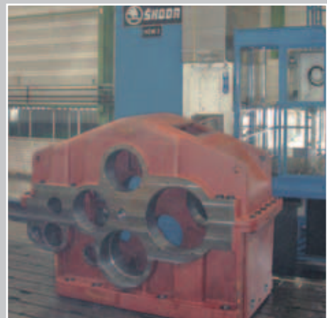
Workstation for machining of large workpieces clamped onto a clamping-plate area.
