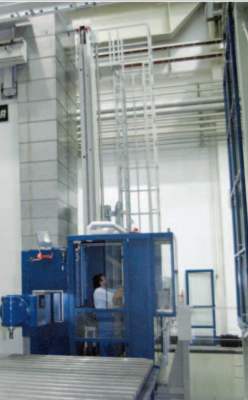
Workstation intended for machining of large crankshaft forgings.
