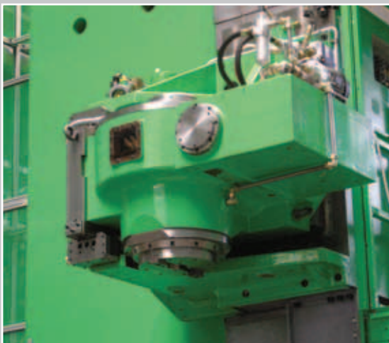
Workstation equipped with special milling accessory to machine turbogenerator rotor slots.
