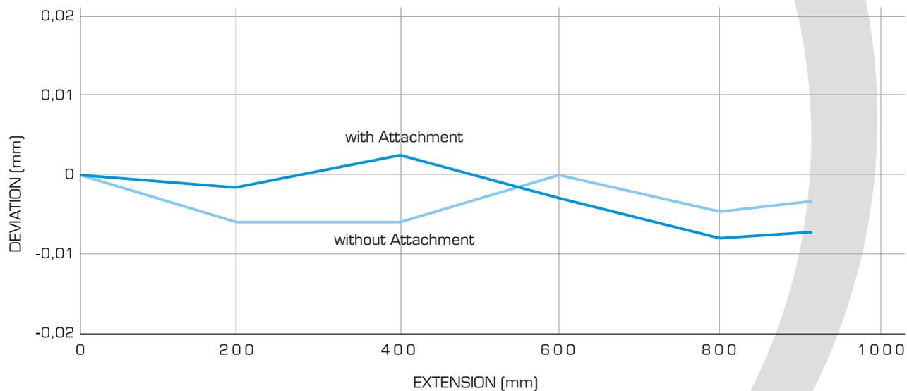
STRAIGHTNESS OF THE SLIDING HEAD MOVEMENT WITH/WITHOUT COMPENSATION
