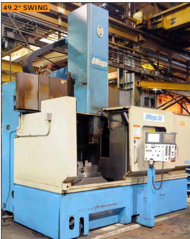
O M LTD. OMEGA 50 CNC vertical boring mill
