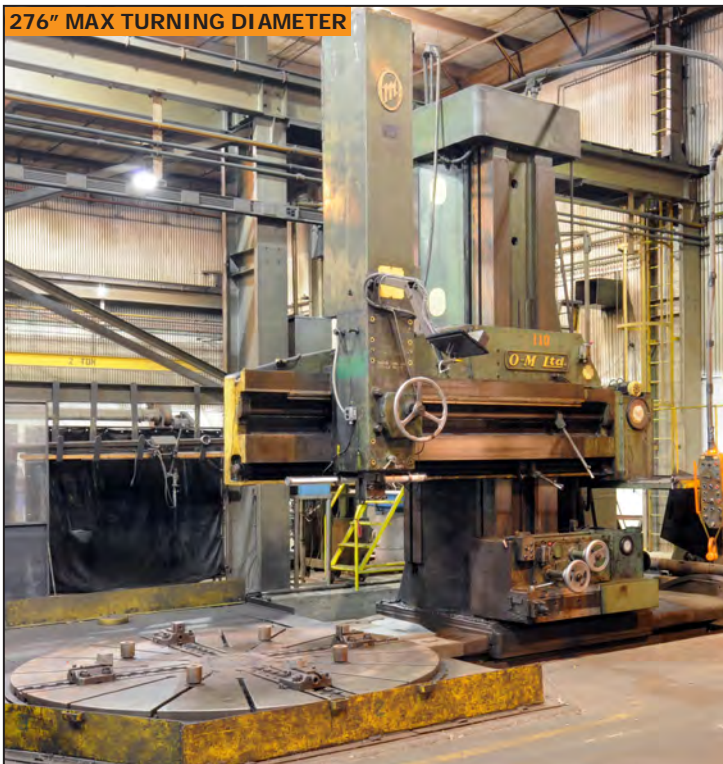
O M LTD. TMS1 30/70 open side and traveling column vertical boring mill
