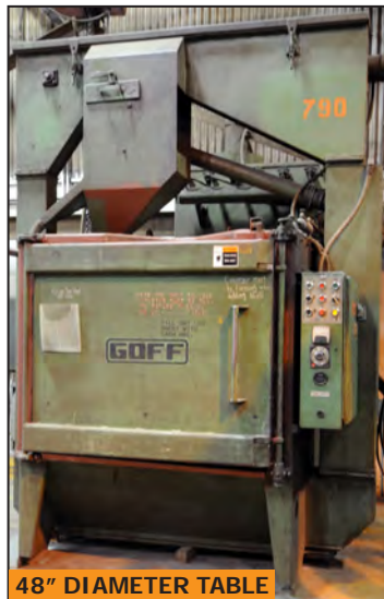
GOFF TB rotary type blast cabinet 48" DIAMETER TABLE
