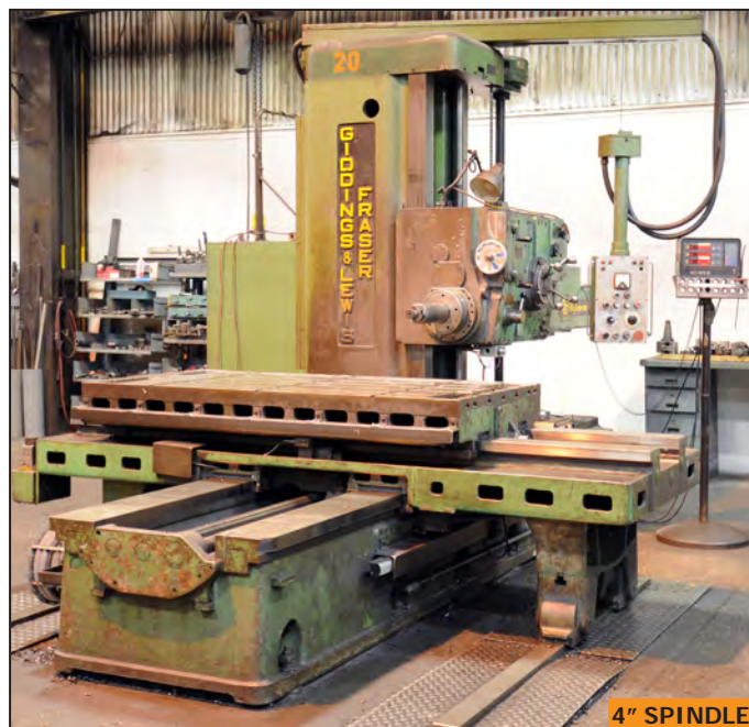
GIDDINGS & LEWIS 70A-DP4-T table type horizontal boring mill
