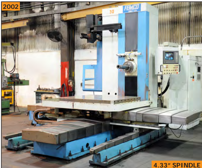
FEMCO BMC-110 R2 CNC table type horizontal boring mill
