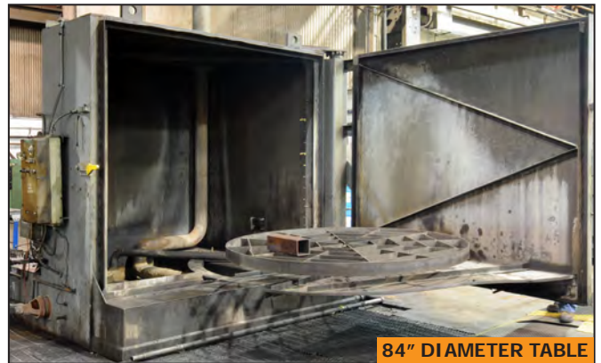
Stainless Steel rotary type phosphate parts washer 84" DIAMETER TABLE
