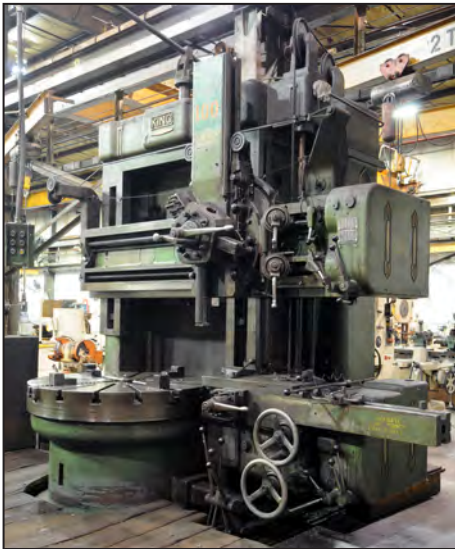
KING vertical turret lathe with side head
