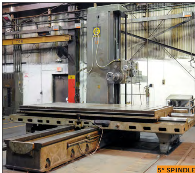
GIDDINGS & LEWIS 70-D5-T table type horizontal boring mill
