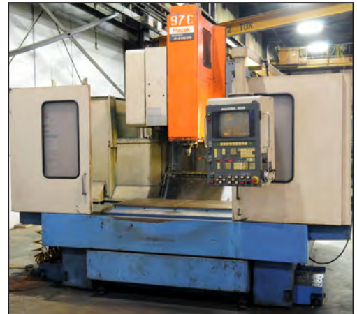
MAZAK V-515/40 CNC vertical machining center
