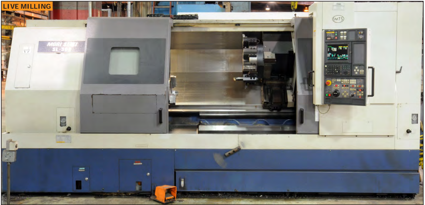
MORI SEIKI SL-303BMC/1500 CNC turning center
