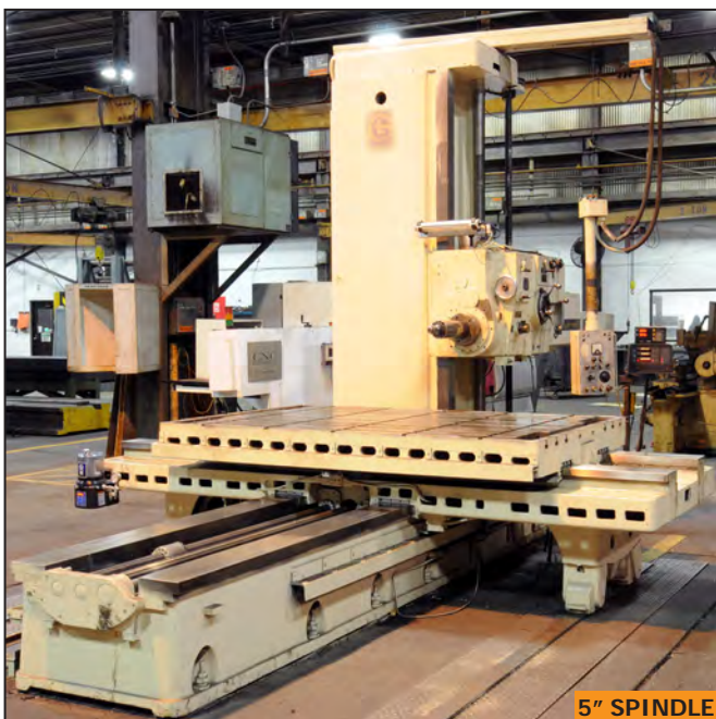
GIDDINGS & LEWIS 65 T5 table type horizontal boring mill
