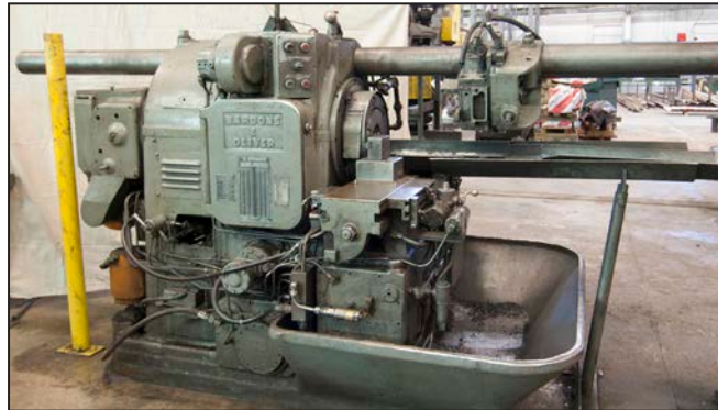
BARDONS & OLIVER NO. 34 cut off machine
