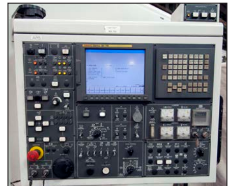
View of FANUC 18i-TB control
