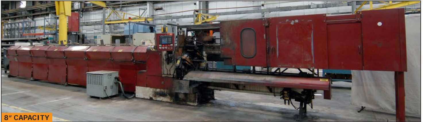
MODERN 8LD cut off machine, ALLEN BRADLEY PLC control, 8" cutting diameter
