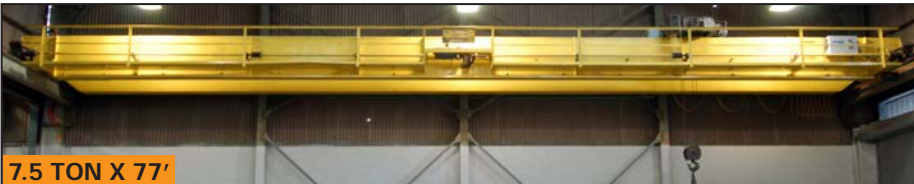
7.5 TON X 77' MANNING MAXWELL & MOORE double girder, top running overhead bridge crane
