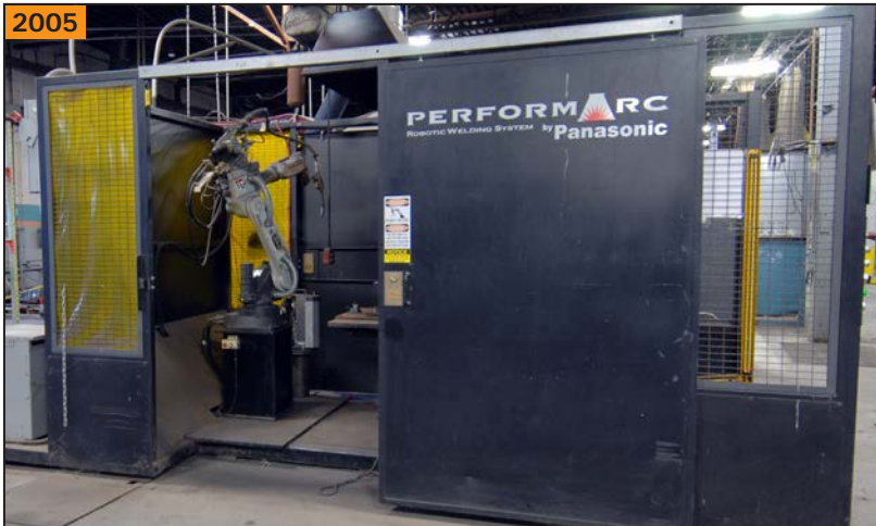
PANASONIC PERFORM ARC 6 axis automated welding cell with VR-006 robot
