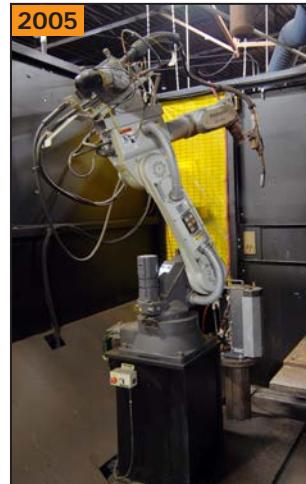
PANASONIC PAR61R1 6 axis welding robot
