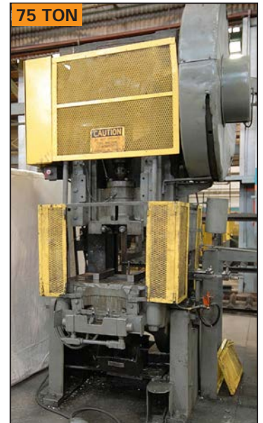
BLISS NO. 23 hydraulic punch press
