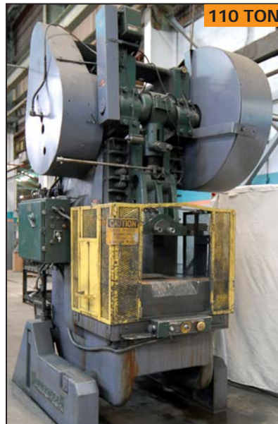
ROUSSELLE MOD # 10 hydraulic punch press
