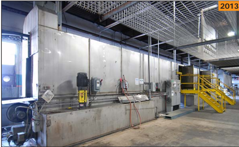
ALABAMA WASHER COMPANY 3 stage overhead conveyor type wash system
