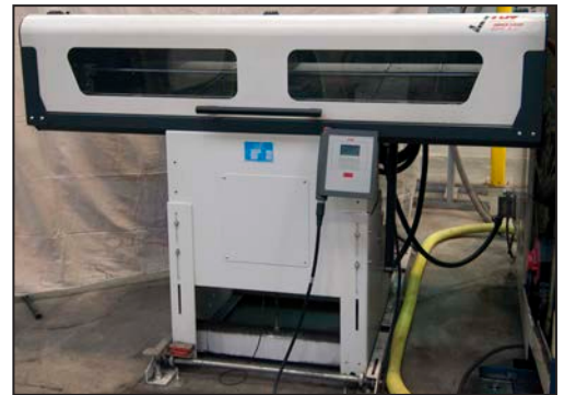
LNS SERVO8052 bar feeder
