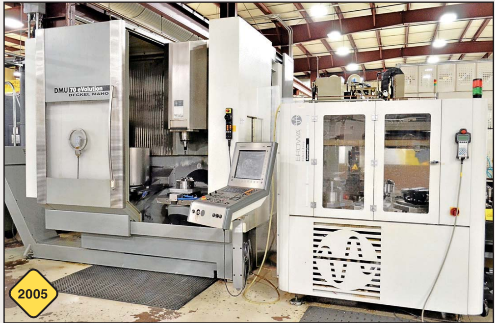
Deckel Maho DMG DMU-70 eVolution CNC Vertical Machining Center, with Erowa Pallet Changer
