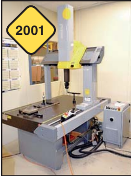
2001 Brown & Sharpe Mistral 07-10-05 Coordinate Measuring Machine
