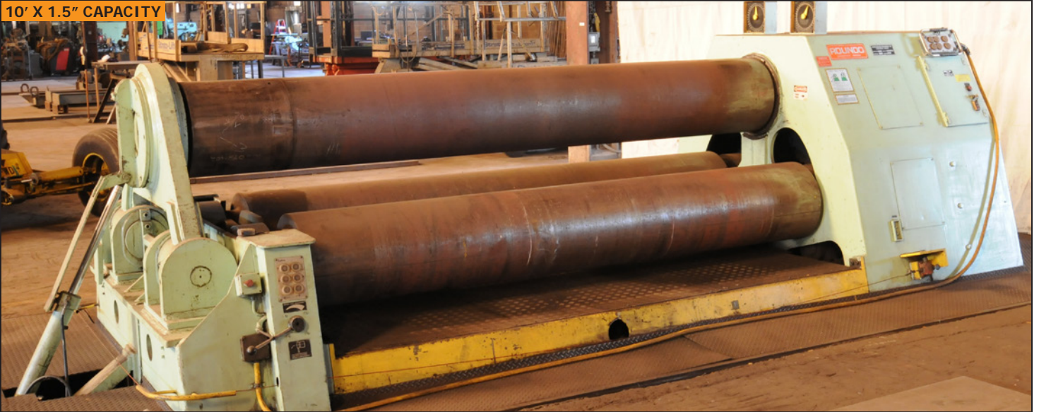
ROUND0 PS 460/10 hydraulic double pinch plate bending rolls
