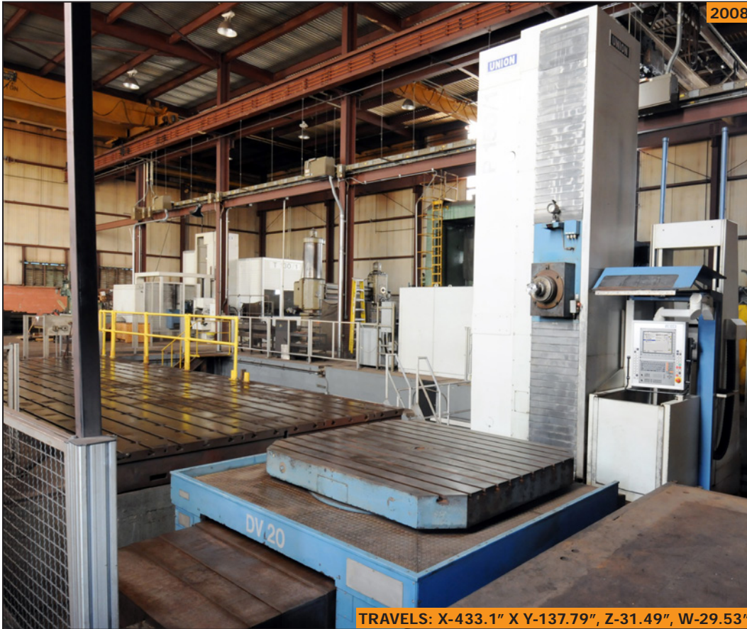
UNION P150/I, 5.9" CNC 7-axis floor type horizontal boring mill with in-feeding rotary table
