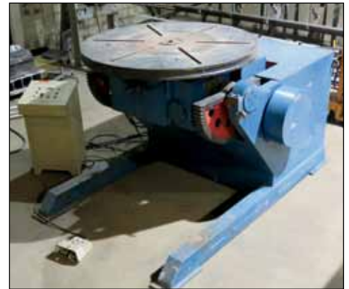
Irizar Mdl. WP-5 Welding Positioner
