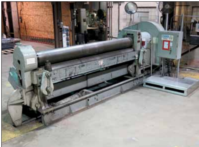
Bertsch 12' x 5/8" Single Pass, 3-roll, Power Plate Bending Roll
