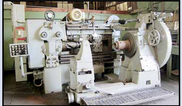
SYKES HERRINGBONE 68" GEAR GENERATOR
