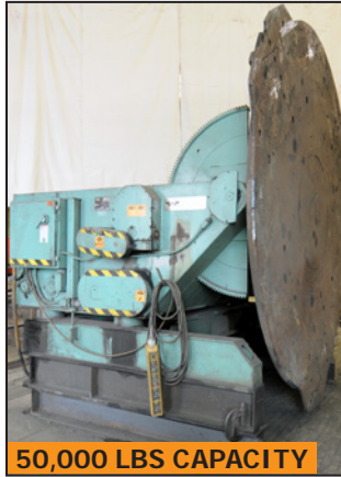
ARONSON GE500CS tilt & rotate positioner w/ geared elevation
