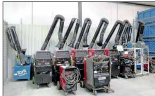
VIEW OF WELDERS AND FUME EXTRACTORS
