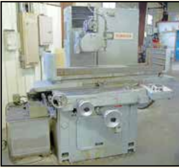
12" x 20" Blohm "Simplex 5" Hydraulic Surface Grinder
