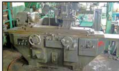
14" x 30" Brown & Sharpe #2 Universal Cylindrical Grinder
