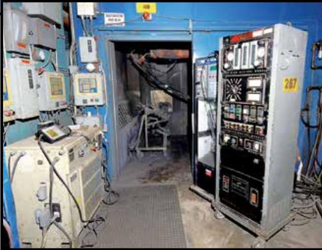
CUSTOM METALLIZING BOOTH #410 , ABB Mdl. IRB6400M98 6-axis robot, Metco 7MC plasma flame control unit w/9MC flow meters, Metco 9MP closed loop powder feed unit, Metco mdl. 9MB gun, Metco 7MR-230 pwr. supply unit, 80 v. DC, 1,100 amp, 100% duty cycle.
