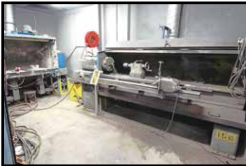
CUSTOM METALLIZING BOOTH #414 : enclosed sound Rockford engine lathe positioner, 80" dist. btwn. centers, 18" swing, front mtd. H.D. travelling torch holder, horiz. metallizing booth w/dual 22" variable spd. rotary tbls. and gas preheaters, Stellite Jet-Koke II Nova D HVOF thermal spray system w/Thermach Mdl. AT1200HPHV powder feeder and JK-3000 SS gun, Metco 7MC plasma flame spray control system converted to 9MC flow meters, 9MP closed loop powder feed unit, Metco mdl. 9MB gun, Metco 7MR-230 pwr. supply unit, 80 v. DC, 1,100 amp, 100% duty cycle.
