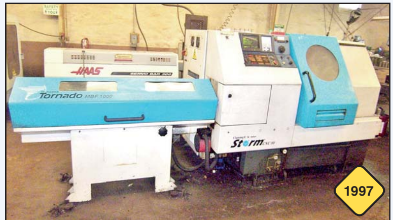
Clausing Colchester Mdl. Storm CNC 80 Lathe, w/Colchester Tornado MBF 1000 Automatic Bar Feed
