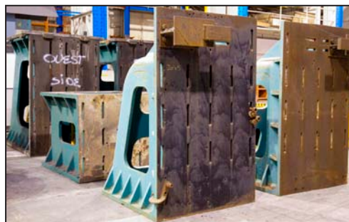
20' x 5' steel angle plates (de-stacked)
