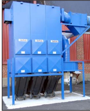
BELFAB dust collector
