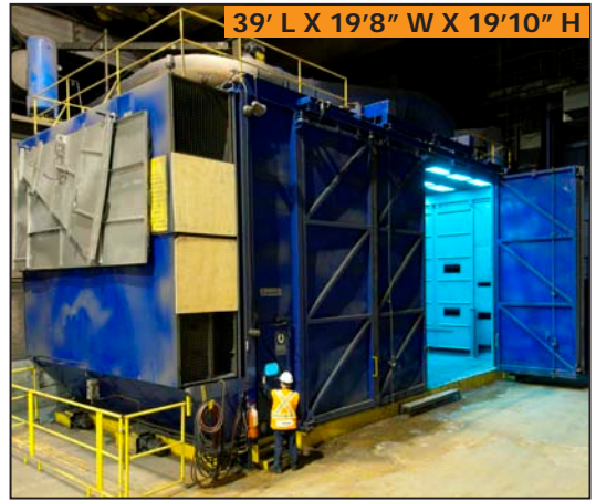
WHEELABRATOR COMMANDER combo shot blast/paint booth
