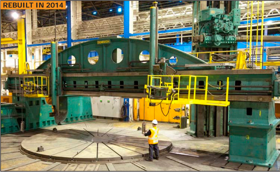
DOMINION 300"/ 504" vertical boring mill
