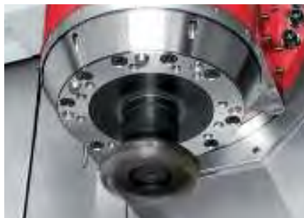
DDS: Direct Drive Spindle
